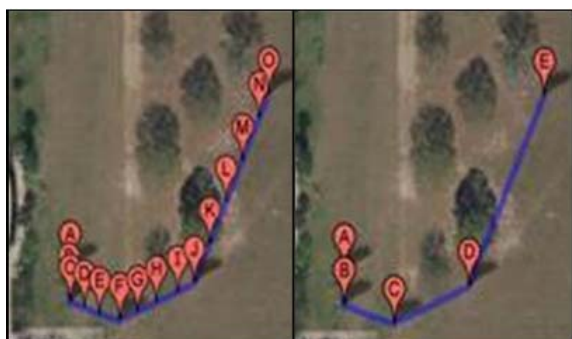
Figure 5 - Trip showing the reduction in points using the Critical Points algorithm.
