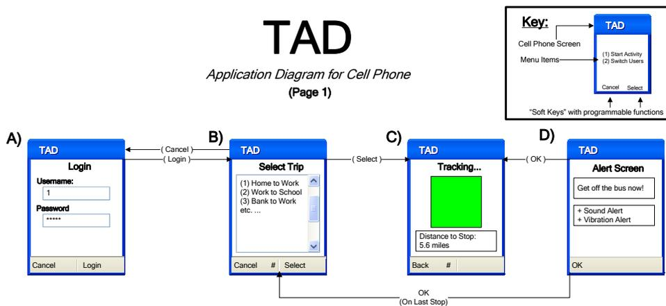
**Figure 3 - TAD Cell Phone Software User Interface**
