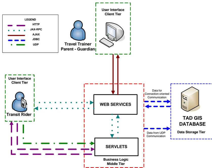
**Figure 2 - Travel Assistant Device System Architecture**
