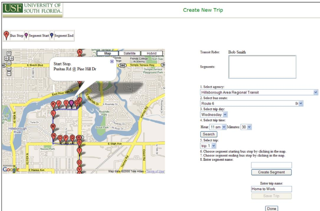
User interface for adding, changing, or deleting transit trip itineraries for uploading to the rider's cell phone for use by the travel assistance device software. The travel trainer or administrator chooses the desired bus route as well as the date and time when the trip will be taken. A single trip may span more than one bus route and involve transfers between buses.
