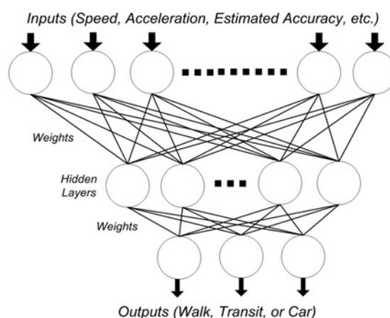
Figure 3 Neural network topology for mode detection
